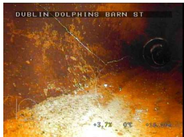
SMH3X_fe378036-504c-4eea-937a-ddab3fadaa73_20220408_102006_609.jpg, 00:05:54, 16.10 m Cracks, radiating from 8 o'clock to 10 o'clock
